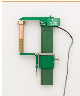
*Model 3565 extensometer for bolt proof load testing*
